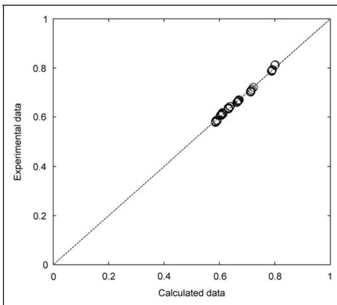
**Fig. 4.** Normal distribution between experimental and calculated flow behavior index by a polynomial model as a function of solid concentration and temperature.
