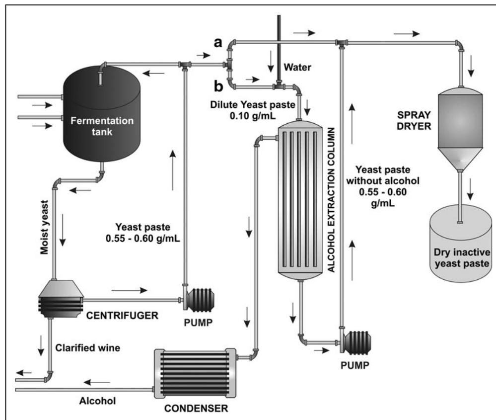
Fig. 1. Process conversion of moist yeast to dry inactive yeast paste.
