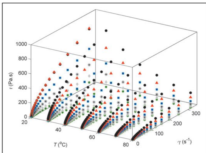
**Fig. 2.** Experimental values of the shear stress of yeast paste as a function of temperature and shear rate at concentrations of 0.15(♦), 0.25(•), 0.35(\*), 0.45(■), 0.55(▲), and 0.64(●) g/mL.
