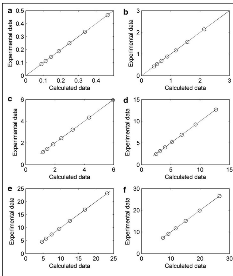
**Fig. 5.** Normal distribution between experimental and calculated flow behavior index of the Power Law model at concentrations of 0.15 (a), 0.25 (b), 0.35 (c), 0.45 (d), 0.55 (e), and 0.64 (f) g/mL.
